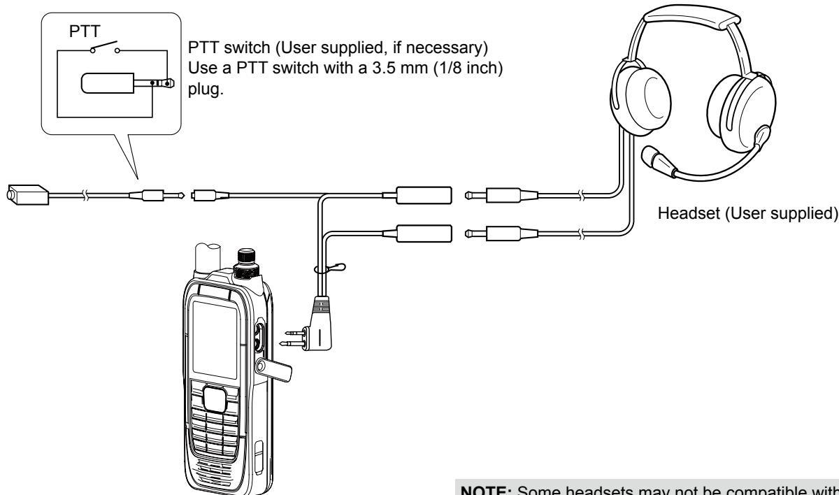
**NOTE:** Some headsets may not be compatible with the transceiver, or need a user supplied adapter to work with the supplied headset adapter. Ask your dealer for details.
