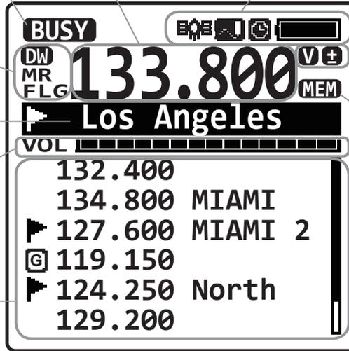
This field displays the icons indicating various statuses of functions, such as “VOX on”, “Split on”, etc.
