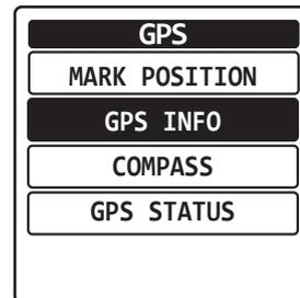
The latitude and longitude of your current position, COG (course over ground), SOG (speed over ground), altitude, and the date will be displayed below the VOL meter on the screen.
