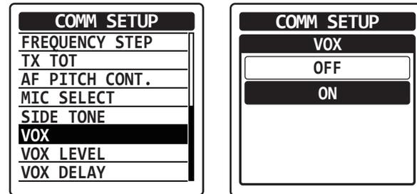
The “**V**” icon, which indicates that the VOX system is active, will appear at the right side of the channel frequency when the display returns to the COM band screen.
