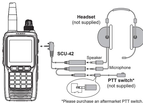
1. Remove the cover and two screws of the **MIC/SP** jack located on the right side of the transceiver.
