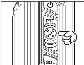
The “**TX**” icon, which indicates that the **FTA-750L/FTA-550/FTA-450L** are in the transmit mode, appears on the display.
